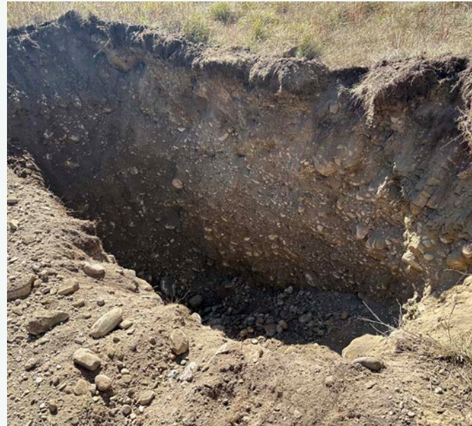
Test pit showing sand and gravel deposits.
