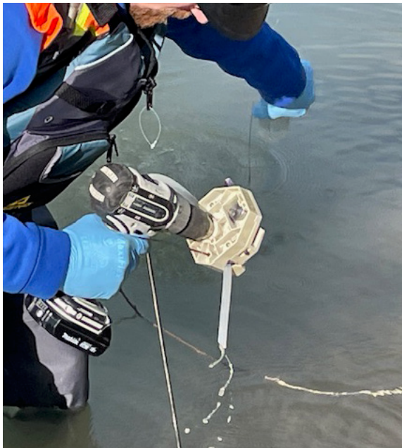
Technician conducts pore water sampling in the ground beneath the stream bed of the Flathead River.
